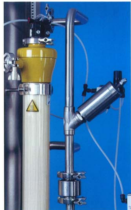
Ultrafilter (patented) and three-stage pressure regulation valve
